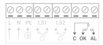
The contact will be closed between the Common (C) and Alarm (AL) points in case of:
